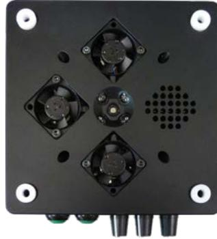
3. Disassemble the punched plate on the bottom side by removing the 4 screws with the hexagonal socket screw key SW 2.0.
